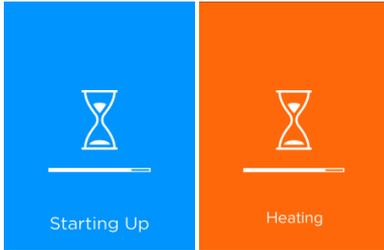
The LCI-777® is typically ready for a breath test in less than 30-seconds. In extreme cold, the device must warm the sensor to a set temperature. This may take up to 2-minutes. The temperature of the sensor and mouth are key factors in alcohol breath testing.
