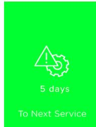
Calibration is required at set intervals established by your monitoring authority. The IID will display a countdown reminder, if you pass the date, the unit will lock out.
